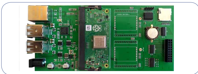
ID CONTROL 500 with two integrated RFID readers (can be installed in access control systems, e.g. in turnstiles)
